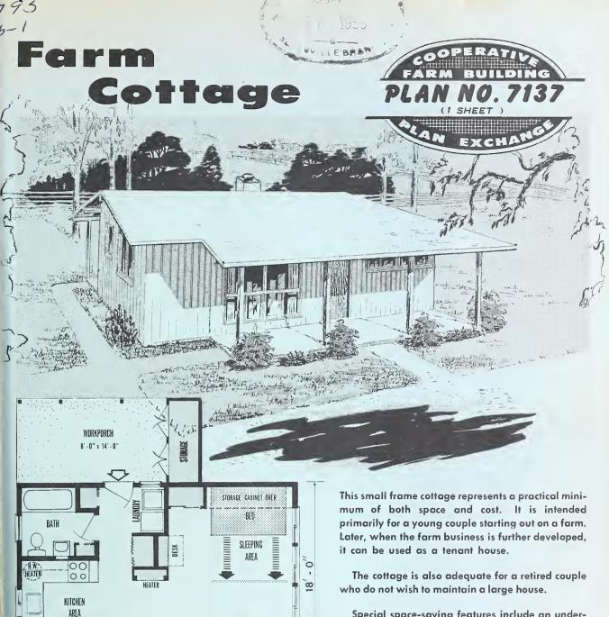
Special space-saving features include an undercounter water heater, a pullout bed, a wall desk, a wall-type heater with a prefabricated metal or asbestos-cement chimney, and accordion-type closet doors.
