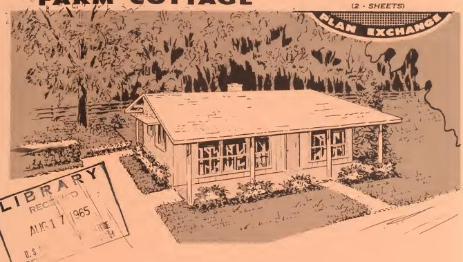
The interior plan of this cottage is the same as that of Farm Cottage, Plan No. 7157. But the roof and window areas have been redesigned, and projecting fixed trellis shades have been added to the east and west windows. With these changes, the cottage can be partly heated by the sun in winter and protected from it in summer.
